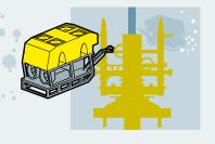
**Condition-based maintenance** of subsea "Christmas tree" assemblies of valves prevents an unexpected breakdown that could result in two days of lost production.
